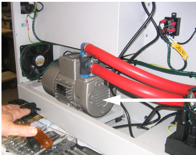
The vacuum pump sits on a tray in the Python casing
